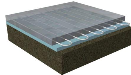
Note: Tube depth is measured from top of embedded layer to the centerline of the tubing.
