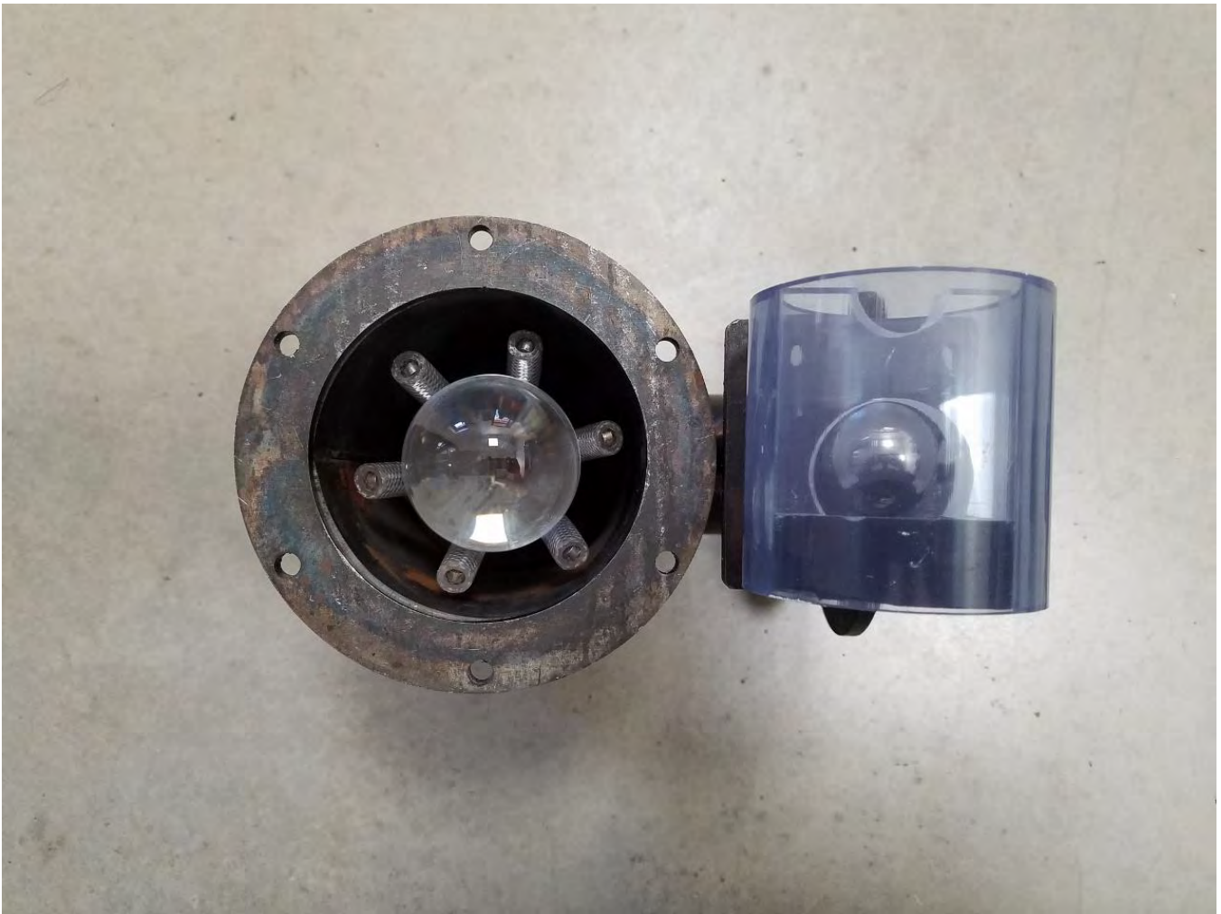
Details of the Pump Clack and Check Valves
